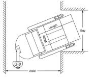
Aisle dimensions listed above assume the minimum bay width to be straddle OD plus 5" (2.5" on each either side of straddle leg). Straddle OD is the load width plus 8". Truck performance may vary due to application requirements' and changes in model design.
